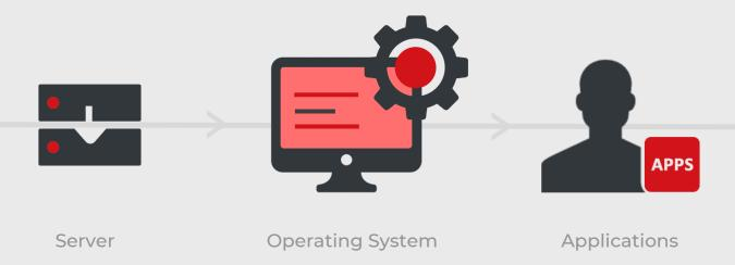
Physical servers allocated to a single tenant. Unlike virtual or cloud servers, there's no virtualization layer—your operating system and applications run directly on the hardware.
